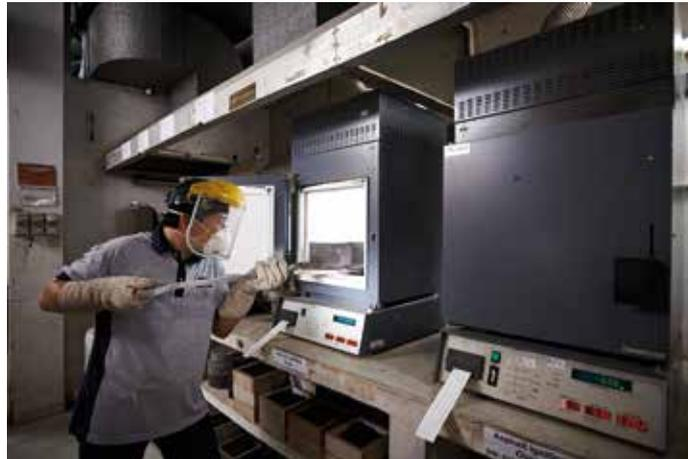
CAST Laboratories Bitumen Content Test determines the asphalt content of a bituminous paving mixture. The test is carried out by placing a sample into an ignition oven and burning off the bitumen. The mass of the remaining aggregate is then weighed and measured.
