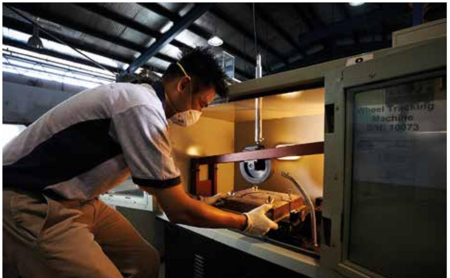
CAST Laboratories Wheel-Tracking Test determines the susceptibility of bituminous mixtures to deform plastically at high road temperatures when under pressure.
